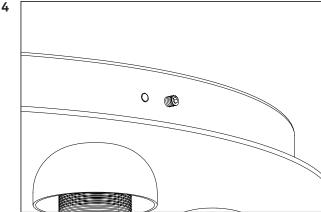
Lock the decorative plate in place by tightening the set screw with the included allen kev.
