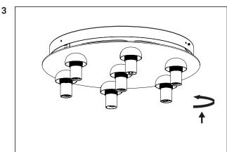
Push the decorative plate up into the ceiling bracket and turn against the clock to fixate in place.
