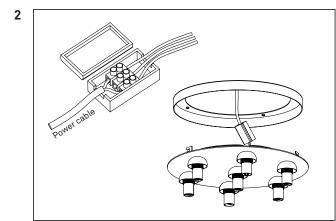
If the power cable is surface mounted make sure to put the cable through the hole in the ceiling bracket before the following,
