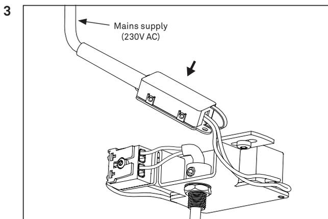
**CAUTION:** Connecting mains supply 230V AC directly to the pendant will damage the LED-module.
