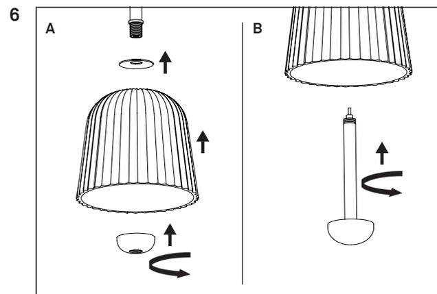
**A:** Lead the curved washer to the ceiling plate. Carefully place the lampshade underneath the curved washer. Place the reflector under the lampshade. Fix it by turning the reflector clockwise.
