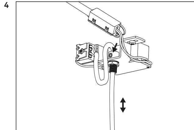
Adjust the height of the pendant by releasing the strain relief and lead the suspension cable through. Retighten the strain relief to secure the height.
