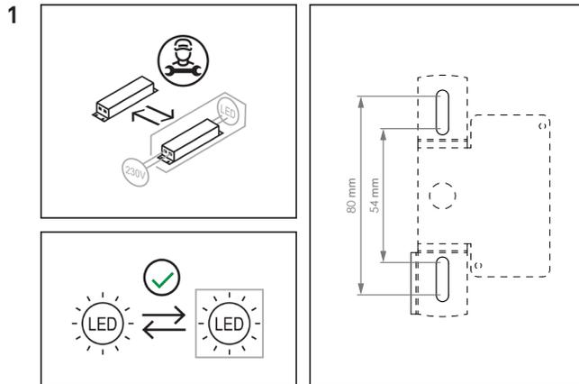
The driver must be replaced by a professional.
