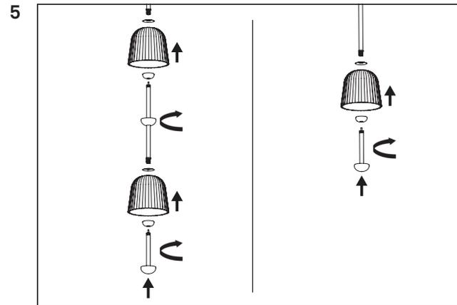
Lead the curved washer through the thread.
