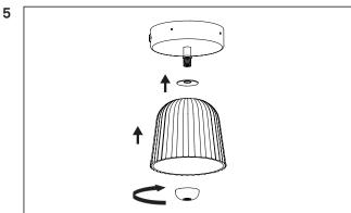
Lead the curved washer to the ceiling plate.
