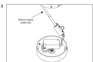
Use the cable terminal inside the enclosed terminal box to connect mains power to the input side of the driver.
