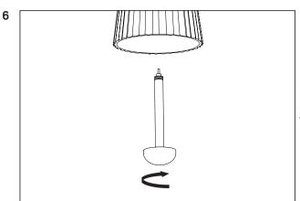
Place the tube under the reflector and fix it by turning the tube clockwise.
