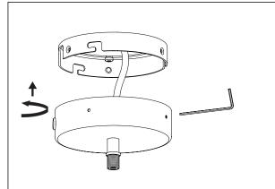
A: Attach the base of the lamp to the bracket by aligning the pins inside the base with the slots in the bracket and twisting the base counterclockwise.
