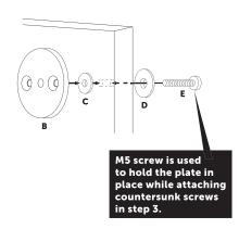
**3.** Attach plate to door with countersunk screws.
