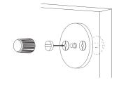
**5.** Attach T-bar to plate with M5 screw. For extra strong fit; hold the screw still with a screwdriver, and tighten the handle by screwing the T-bar by hand.
