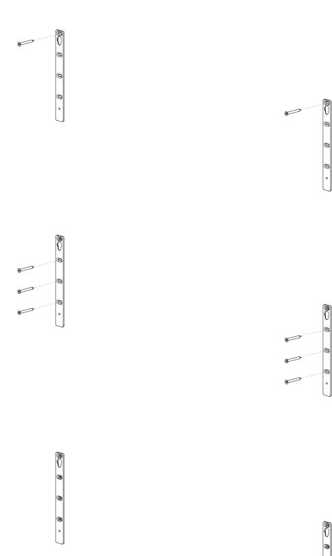
a. Screw in two screws in the top mounting holes on both bracketsDo not fully tighten down
