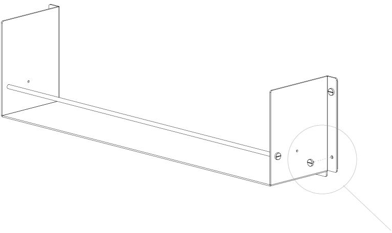
Tighten the bottom coin screw on both sides.
